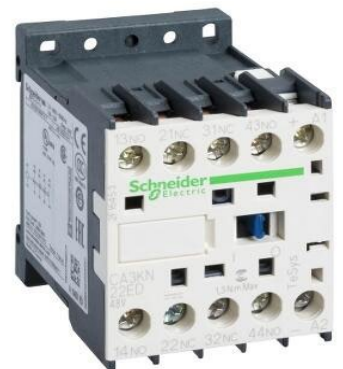
SCHNEIDER ELECTRIC CA2KN31E7 TESYS K CONTROL RELAY 3 NO + 1 NC <= 690 V 48 V AC COIL 3389110500356
