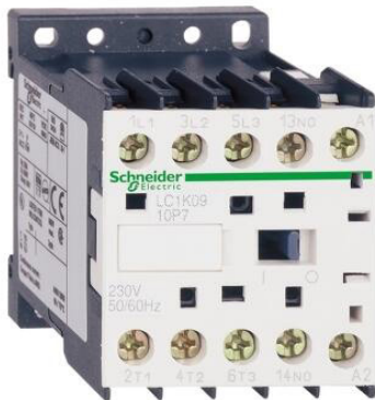
SCHNEIDER ELECTRIC LC1K0901Q7 TESYS K CONTACTOR 3P(3 NO) AC3 <= 440 V 9 A 380...400 V AC COIL
