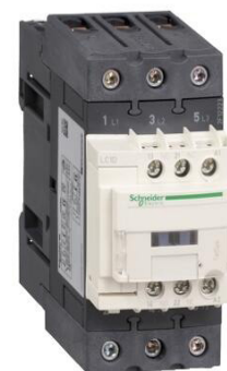
SCHNEIDER ELECTRIC LC1D50A- ED TESYS D CONTACTOR 3P(3 NO) AC3 <= 440 V 50 A 48 V DC STANDARD COIL 3389119408790
