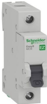
SCHNEIDER ELECTRIC EZ9F51140 1X40A 10KA 230V TYPE C EASY9 AUTOMATIC FUSE 3606481201751
