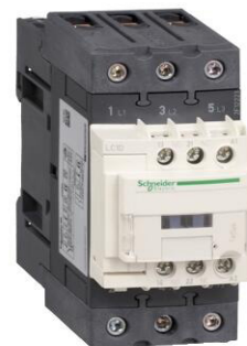
SCHNEIDER ELECTRIC LC1D38FD TESYS D CONTACTOR 3P(3 NO) AC3 <= 440 V 38 A 110 V DC COIL 3389110359923
