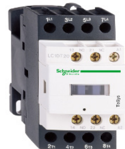
SCHNEIDER ELECTRIC TESYS D CONTACTOR 4P(4 NO) AC 1 <= 440 V 25 A 220 V AC COIL 3389110577679
