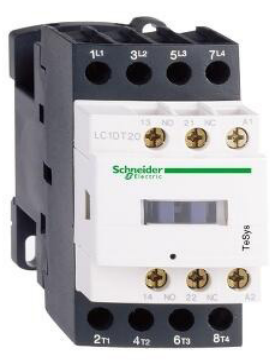
SCHNEIDER ELECTRIC LC1DT32BD TESYS D CONTACTOR 4P(4 NO) AC1 <= 440 V 32 A 24 V DC COIL 3389110247824
