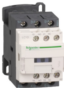
SCHNEIDER ELECTRIC TESYS D CONTACTOR 3P(3 NO) AC 3 <= 440 V 12 A 230 V AC COIL 3389110349306
