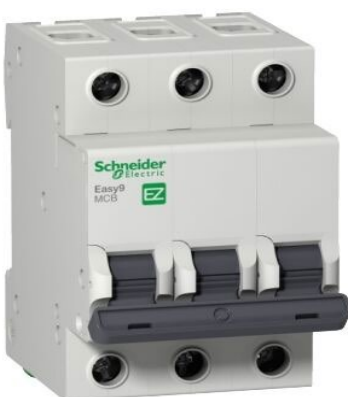
SCHNEIDER ELECTRIC EZ9F56363 3X63A 6KA 400V TYPE C EASY9 AUTOMATIC FUSE 3606480587887
